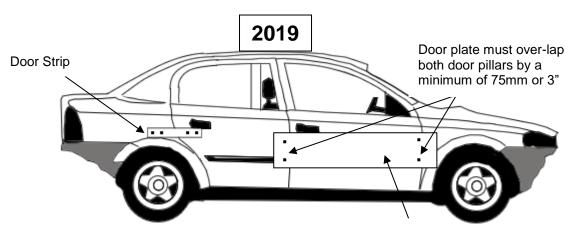
The Door plate must be fixed by either four 19mm bolts or studs, or six 13 mm bolts or studs, through both the door pillars. No slotted holes allowed
